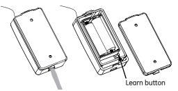
**Step 2** - Press and hold the Learn button inside the Silent Alert. One of the LED indicators on the front of the Silent Alert will begin to flash.
